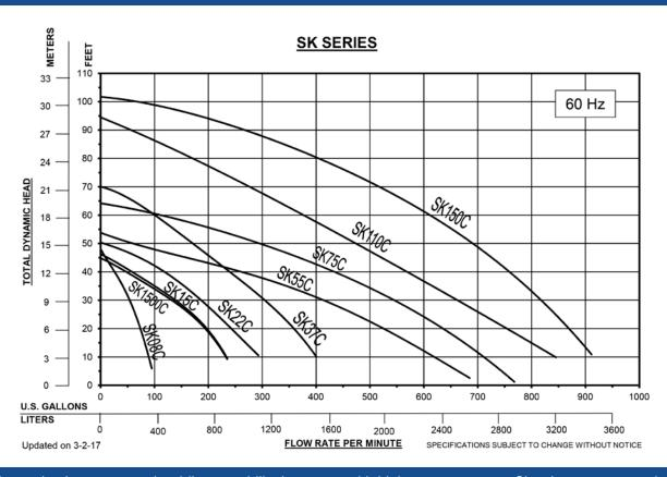
Note: When selecting a pump, shredding capability increases with higher motor torque. Size the pump to apply as much motor HP as possible. For optimal performance, the pump must be sized correctly for the application.
